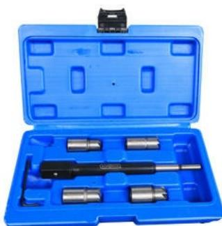
**FRESA PARA ASIENTO DE INYECTOR DIESEL**
